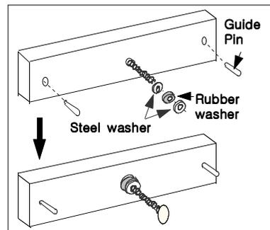
Fold the mounting Template along the dotted line to a 90-degree angle. Make sure the Hole Guide Pins are in the two guide pin holes. Put on rubber washer between two steel washers, and place them over the armature screw between the armature plate and the door.
